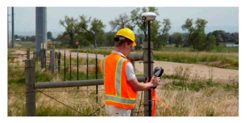
Well Location Survey: For the development of new well locations or the mapping of existing well locations. Marks the location of a well site in relation to the unit lines or survey lines.
